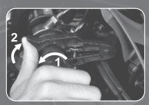
2: Reach desired speed and engage EASY CRUISE by rotating clockwise to rest over the break lever.
