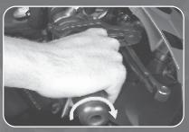
3: Disengage by twisting the throttle lock clockwise or forward as you normally reduce the speed.
