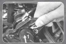
1: Slip on silicon ring and then slip on EASY CRUISE over the silicon ring from top or side of the throttle. Make sure front bottom flat surface of EASY CRUISE should cross over the front side of the break lever by few mm. Adjust tension gear for suitable Friction.
