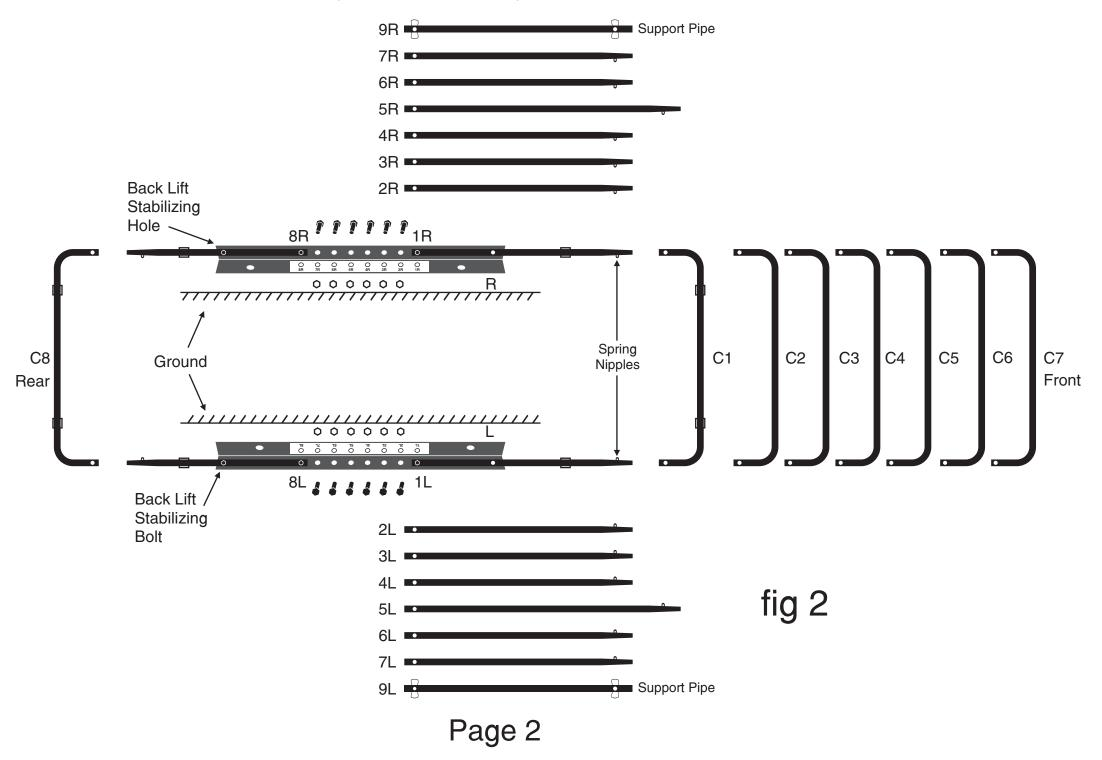
STEP 3 : Snap the C tube C1 & C8 (with attached legs facing down) to the corresponding L & R tubes of #1 & #8, make sure that C tube should be inserted evenly on L & R side tubes to avoid a jam. Once inserted you will have to press the nipple installed at the end of each straight tube and push C tube till you hear a click and nipple comes through the hole of the C tube (As shown in fig. 3(A)).
