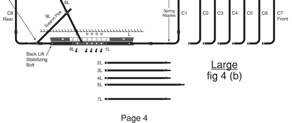
STEP 5 : Attach the balance straight tubes (L & R Sides) by using provided bolts & nuts to the corresponding holes on the "L" Bracket (Note : straight tubes should be connected on inner face of "L" Bracket)
