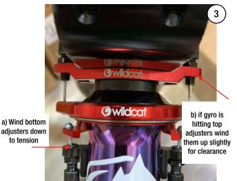
a) Wind the bottom barrels out / down to add some tension the bottom cable assembly. Wind top barrels up only if the gyro hits them and clearance is needed. Again we want to have as little tension above the gyro as possible.
