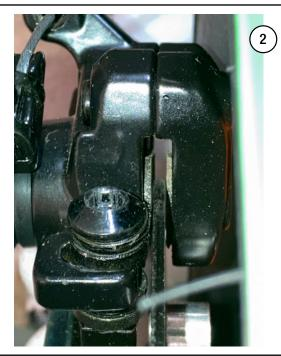
a) Align brake on disc (mount, two x 5mm hexes ensuring the wheelside pad is as close as as possible to the disc without touching. Spin to make sure it doesn't rub.
