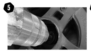
Flip the wheel over, and push down on the tyre / rim against the floor, the hub will simply slide out of the rim assembly.
