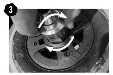
Wind the collar off the hub. Insert the hub assembly into the rim, valve side up (It will only fit one way). You will need to rotate back and forth as you push inwards to clear the inner flanges.
