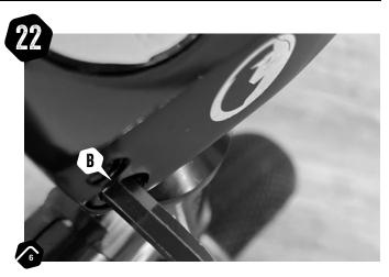
Once the bars are correctly aligned with the wheel and there is no play in the head parts / forks (bars must still turn freely), secure the pinch bolts tightly with a 6mm allen key.
