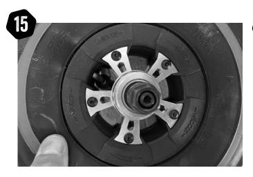
Once the spacing is relatively even, fully inflate to the required pressure (35-45psi for Cross wheel).
