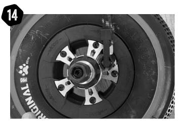
As per the TURBO WHEEL instructions - Partially inflate, just so the tyre lightly grabs the rim. Take note of the bead line around the tyre close to the rim edge. For balance you want the space between this and the rim to be even the whole way around on both sides.
