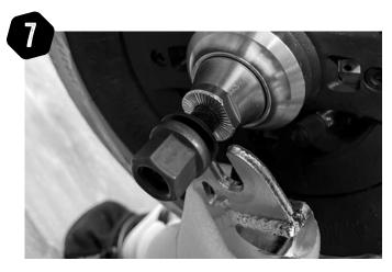
Place bike upside down, insert assembled wheel axle into the fork dropouts. Wind the axle nuts in by hand at first. **IMPORTANT:** ensure the keyed washers insert into the triangle holes on the dropouts.
