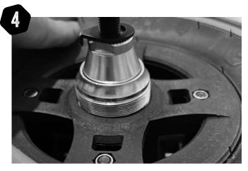
Flip over, then push down firmly on the wheel against the floor to correctly seat the hub in the rim assembly.
