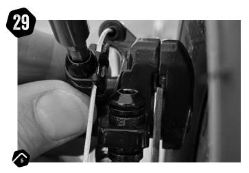
Push the arm forwards until the outside brake pad almost touches or lightly touches the brake pad. Tighten the cable clamp using a 5mm allen key. Then squeeze the brakes firmly a few times, this will settle the cable and back the adjustment off slightly. Before testing, spin the wheel and check if there is any disc contact. If so, undo the cable clamp and back the arm off slightly then re-tighten.
