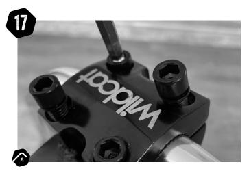
Lightly tighten down two diagonally opposite until it begins to pinch on the bars. Then rotate the bars up and tighten slightly more to hold them in place.
