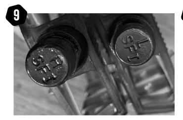
Pedals are marked 'L' & 'R' on the end of each spindle. OG has a 1 piece crank and 1/2" thread pedals, OG-PRO has a 3 piece crank with 9/16" pedals.
