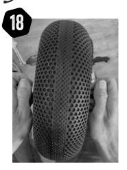
To check balance, hold up the wheel and spin. You may see a light visible wobble but as long as you cannot feel it in your arms it will run smooth. If it feels off balance check the bead line against the rim both sides as it spins to gauge where you need to adjust. Deflate and repeat.
