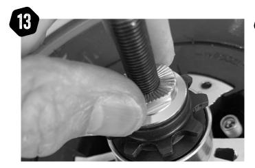
Replace the spacer and wind down to hold the assembly in place. Once together visually check the large spacer between the hub halves is correctly seated in both sides. It will have a little slop until you tighten down the 5 x 3mm hub bolts.
