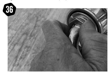
Adjust the bearing cone as required, (this is also reverse thread) semi retighten the 32mm locking nut anticlockwise and spin to check again. Repeat if further adjustments are required, then tighten securely.
