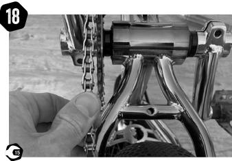
Replace the wheel back onto the frame and loop the chain back onto the chainwheel. Tighten axle nuts by hand at first to align wheel and tension chain, then fully tighten. Check alignment of disc brake and adjust if required.
