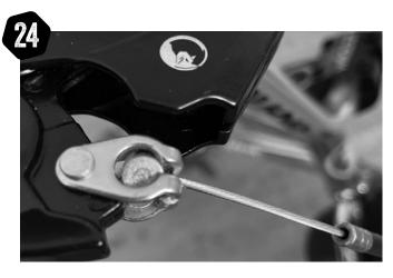
Squeeze the lever to expose the cable clip and insert the round cable head as shown.
