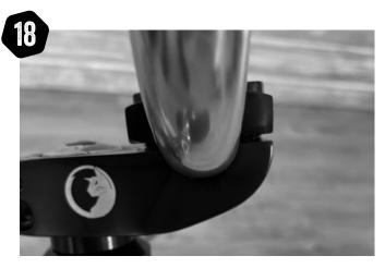
Check from the side to ensure the stem plate is parallel with the stem, the gap both sides should be equal. If not, back off the low side and slightly tighten the other.
