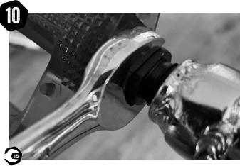
Carefully insert the 'L' pedal on the left side and start to wind in by hand. Then using your 15mm spanner, (remember it is reverse thread! turn anticlockwise) and tighten. Make sure you do it up nice and tight, loose pedals destroy thread fast!
