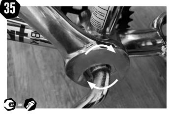
If adjustment is required back the 32mm nut off with a spanner or wrench. This is reverse thread, so clockwise to loosen.
