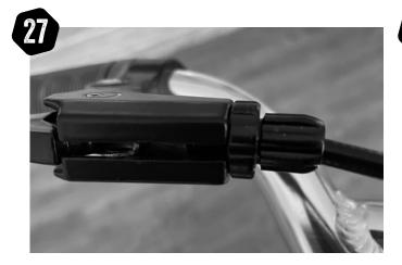
Tighten the cable adjuster barrels against the lever, ensuring to misalign the slots to prevent the cable escaping.
