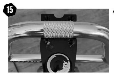
Undo the 4 x bolts with a 6mm allen key and remove the stem plate. Ensuring all contact surfaces are clean from grease or dust, place the bars centred in the stem with the brake lever to the right side, and hang them down in front.
