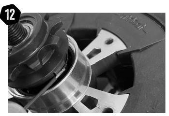
If the driver did pop out, place it back on the axle and holding the 3 x palls in gently rotate and push it back in.
