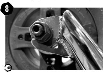
Once they are positioned correctly, fully tighten the axle nuts with a 15mm spanner.
