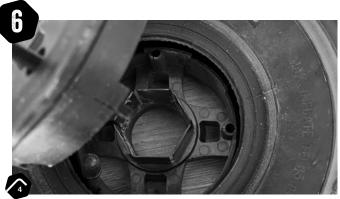
**NOTE: ENSURE THE TYRE IS DEFLATED BEFORE CONTINUING.** Undo the 4 x rim bolts using a 4mm allen key, then the rim will simply pull apart off the tyre.
