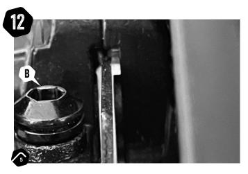
View down the back of the disc. Align the brake and tighten down **B)** the 2 x hex bolts with a 5mm allen key. Ensure there is enough clearance both sides so the disc does not rub. If there isn't enough clearance, the inside brake pad can be adjusted back by removing the rear wheel to access the 5mm hex adjuster on the back of the brake closest to the wheel.
