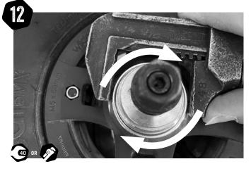
Wind on the collar by hand until it is against the rim assembly. Using a wrench or spanner gently tighten 1/8 - 1/4 turn to ensure the hub is seated firmly and there is no play. CAUTION: Do not over-tighten.
