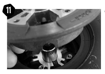
Replace the driver side onto the axle, again check to see the valve slot on this side is aligned correctly.
