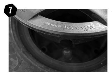
When reassembling, ensure the valve holes are lined up with the valve and it is oriented on the driver side.
