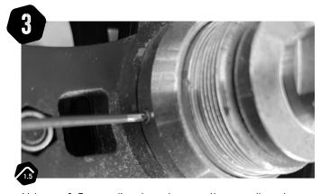
Using a 1.5mm allen key, loosen the small grub screw on the aluminium collar. This collar holds the rim onto the hub assembly.
