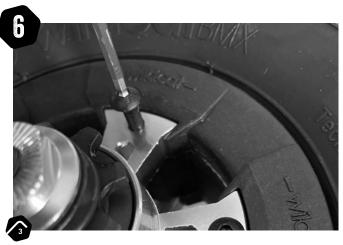
Using a 3mm allen key remove the 5 x hex hub bolts on the driver side only.
