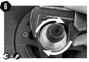
Wind the collar on by hand until it is against rim assembly. Using a wrench or spanner gently tighten 1/8 - 1/4 turn to ensure the hub is seated firmly with no play. **CAUTION: Do not over-tighten.**
