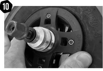
As per removing the hub assembly - flip over, then push down firmly on the wheel against the floor to correctly seat the hub in the rim assembly.
