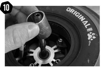
Take care to replace the large spacer and check it's seated correctly before reassembly.
