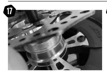
Put the cap back on the valve, and wind the disc back onto the mount firmly. Braking action will further tighten the disc, so only needs to be tight enough to prevent it dislodging during assembly.
