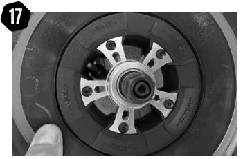
Once the spacing is relatively even, fully inflate to the required pressure (40-50psi for Turbo wheel).
