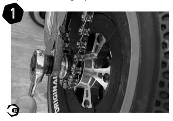
Loosen the axle nuts on both sides with a 15mm spanner.
