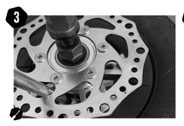
Removing the disc is not 100% necessary, but it does make life a bit easier when inflating and balancing the tyre. The disc is simply threaded onto the hub and is self-tightening when brakes are applied. To remove insert a strong screwdriver or similar through the disc and carefully lever against the back of a spoke (so as to not mark the front).
