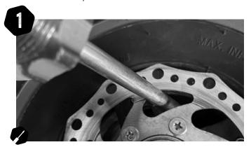
The disc is simply threaded onto the hub and is self-tightening when brakes are applied. To remove insert a strong screwdriver or similar through the disc and carefully lever against the back of a spoke (so as to not mark the front).
