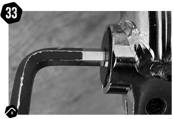
Check and tighten the spindle bolts on the crank axle on both sides with a 6mm allen key.
