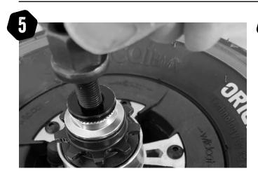
NOTE: ENSURE THE TYRE IS DEFLATED BEFORE **CONTINUING.** Remove the axle nut on the driver side only.
