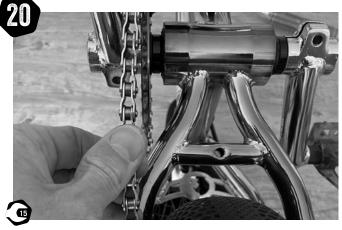
Replace the wheel back onto the frame and loop the chain back onto the chainwheel. Tighten axle nuts by hand at first to align wheel and tension chain, then fully tighten. Check alignment of disc brake and adjust if required.
