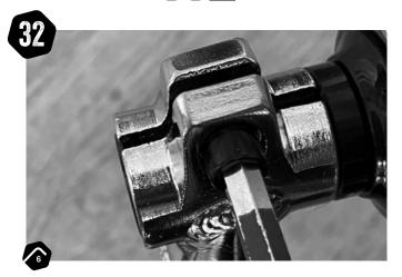
Check and tighten the pinch bolts on the crank arm on both sides with a 6mm allen key.
