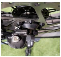
Note: if your bike has a bolt-on front wheel, make sure the nut and washer are on both ends and tighten them with a 15mm hex wrench
