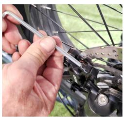
If it sounds like the wheel is rubbing, loosen the caliper adjuster bolts and try squeezing the brake lever again to center the calipers. If it looks like the disc is not centered between the calipers, you can gently push the caliper over with your thumb or finger until it is centered over the disc. Tighten the caliper adjuster bolts and release the brake lever
