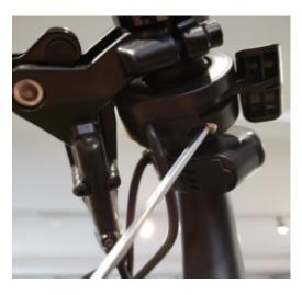
10 Make sure there is sufficient space between the throttle and the brake lever so the throttle does not get stuck
