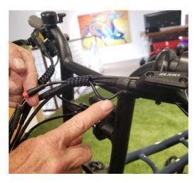
10 If unplugged, connect the cables - red to red. Make sure the pins and notches are lined up, arrow to arrow
