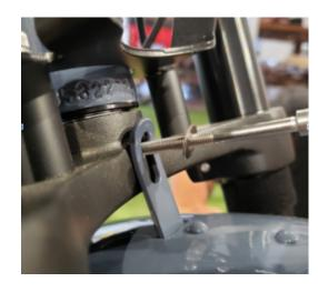
8 Angle the fender so it is nice and even over the tire
