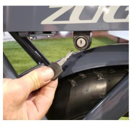
4 With the key turned, use the handle under the bottom of the battery to pull it out
