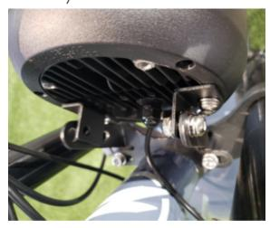
6 Tighten both bolts down. You can use a 10mm or your finger and a 4mm allen
