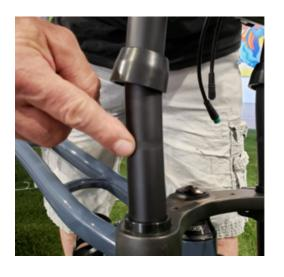
3 With a 5mm allen key tighten the two allen key bolts on the side of the fork. To tighten, turn each bolt 1-2 circles to the right, alternating bolts
