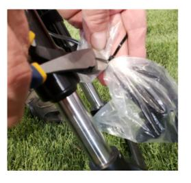
6 Pull the black plastic tab out of the brake caliper
