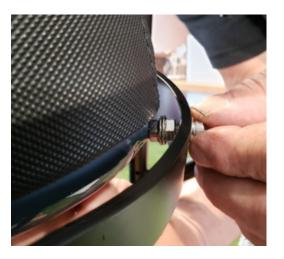
8 Using the 8mm hex and 4mm allen tighten down the main bolt
