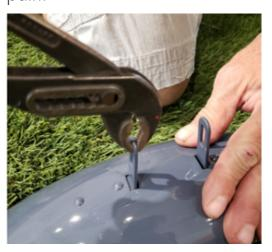
4 Squeeze the back mount closer to the front by hand or using the corner of a table or bench.
