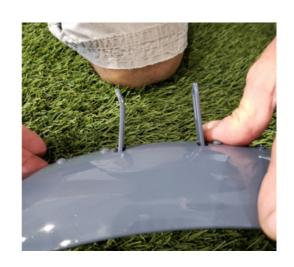
5 With the mounts moved in closer, it should then fit snugly against the fork crown. If not, no worries, you can always bend it in a little more!
