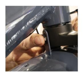
6 Insert the bolt and the washer into the front side of the fender
