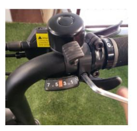
8 To adjust the keypad's position, use a 2.5mm on the backside of the keypad. Tighten (ignore the strange sound!)
