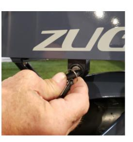
2 Insert the key into the lock cylinder located on the left side of the bike under the battery tray
