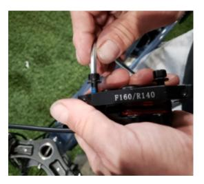
7 With your 4mm wrench, tighten the two rotor adapter bolts
