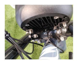
7 Locate the headlight plug (reddish/orange). Line up the arrows, notches, and pins, and connect the two sides together (gently!)
