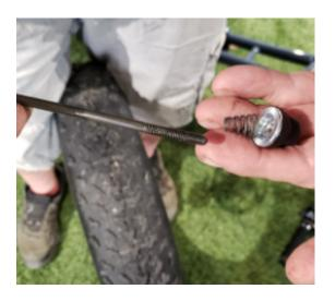
12 Flip the wheel around, and on the disc side, slide the spring onto the bolt with the larger part of the cone facing towards the outside of the bike and screw the cap on
