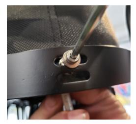
10 Tighten the smaller side bolts and then slide your battery back in and ensure it is locked. You're all done!
