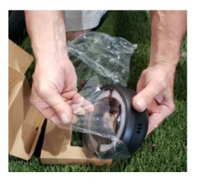
2 Remove the 2 screws, washers, and nuts from the bracket part of the headlight and set aside
