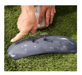
3 Bend the front mount slightly with a pair of pliers to bring it away from the headtube of the bike, so that it doesn't try and scratch the paint
