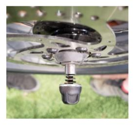
15 While holding the non-lever end of the quick release bolt steady with one hand, screw the quick release lever to the right with your other hand. Tighten it until it is HARD to close. Flip the lever into the "close position"
