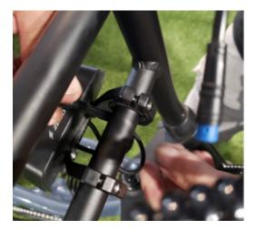
7 Connect the display cables - green to green. Make sure the pins and notches are lined up, arrow to arrow
