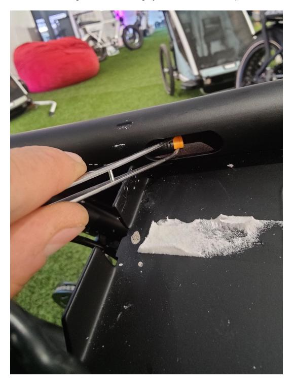
Inspect the pins on the plug and make sure the male and female sides look good before reconnecting, always align the two arrows, never force the cables, and always press them together firmly.
