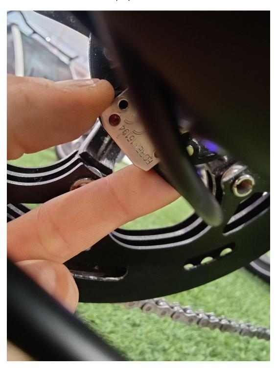
Reinstall the screws to attach the PAS to the mount
