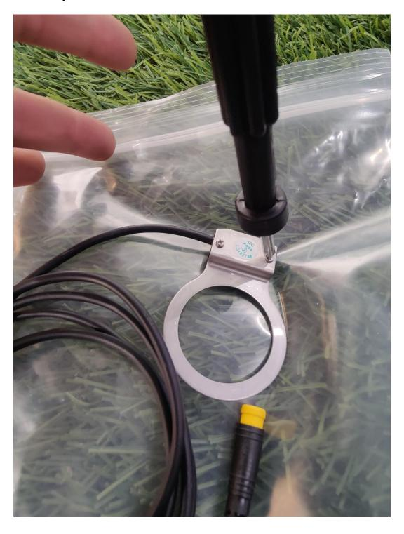
Feed the Julet end of the sensor into the bottom of the frame and begin feeding it up so the hole that it was previously located.
