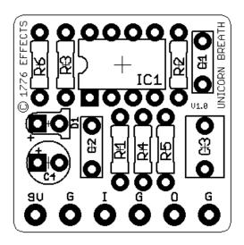
The "Unicorn Breath" buffer is based of the famous pedal that rhymes with thon. A few modifications in my design include a buffered bias voltage and the use of a particular dual opamp, the OP275. This opamp was chosen for it's exceptional transparency, although other dual opamps can be used with good result.
