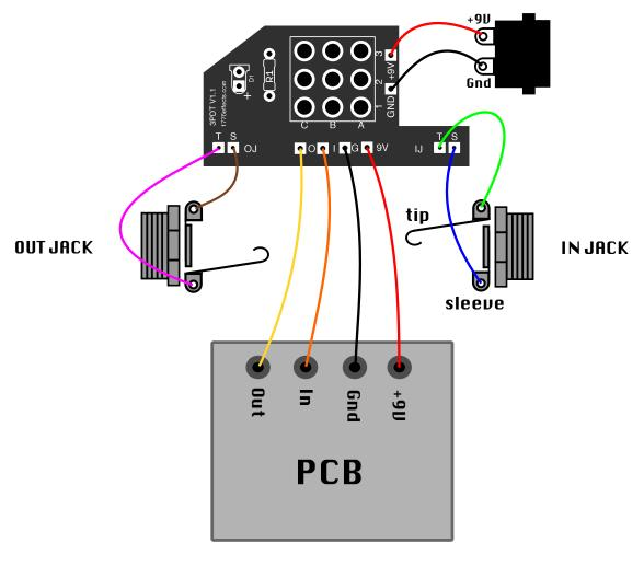
R1 - Current Limiting Resistor for LED D1 - LED
