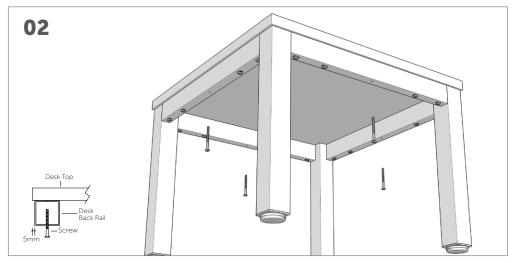
Fix worksurface with 5mm overhang to frame, then fully tighten all rail to frame screws.
