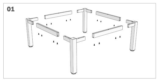
Assemble frames and rails together, loosely (1 turn from tight).
