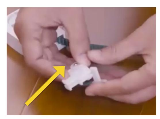
Don't put the runner wheel in the wrong way around, buckle first wheel nearest the endcap
