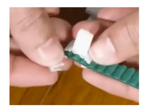
5. Remove the buckle from the ribbon and remove the 2nd runner wheel and buckle
