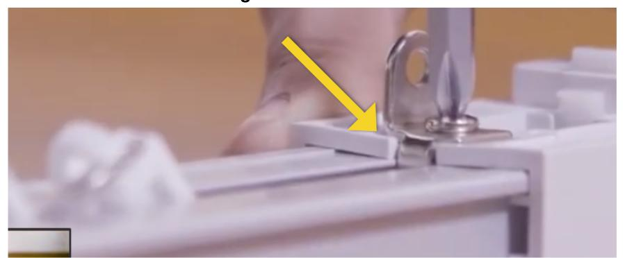
9. Use the Distance between the endcap and track to finetune the tension and easy movement of the assembly
