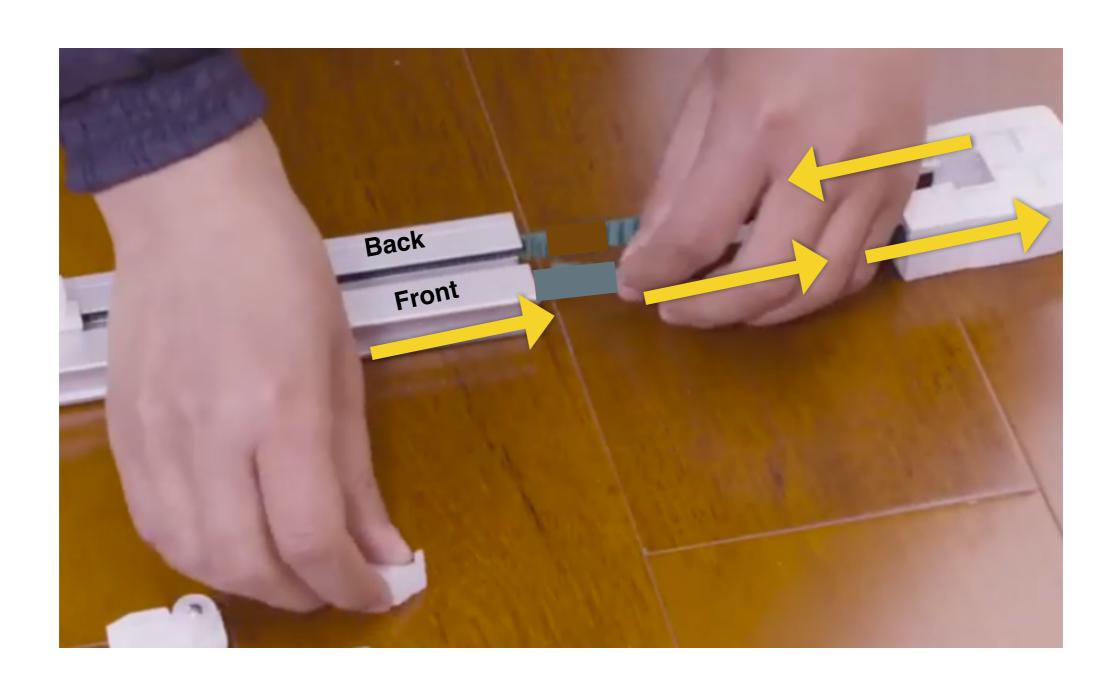
8. Where before the Buckle was in the front of the track, it will now be assembled and run the back of the track, thus reversing the direction of Open and Close
