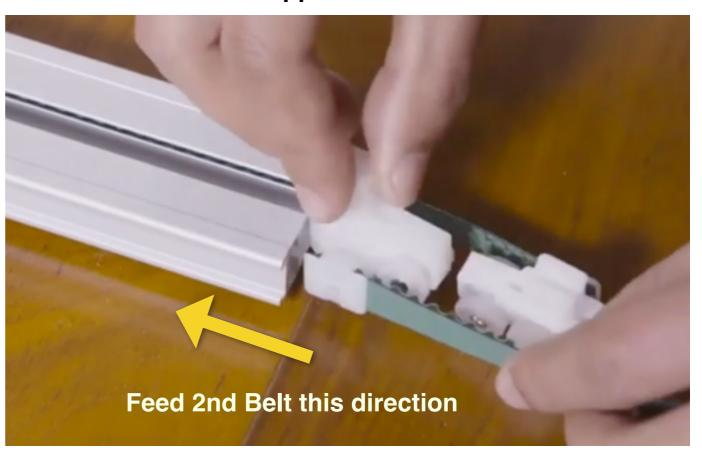
11. Feed the belt through the track end, make sure the wheel opening on the track end cap faces up
