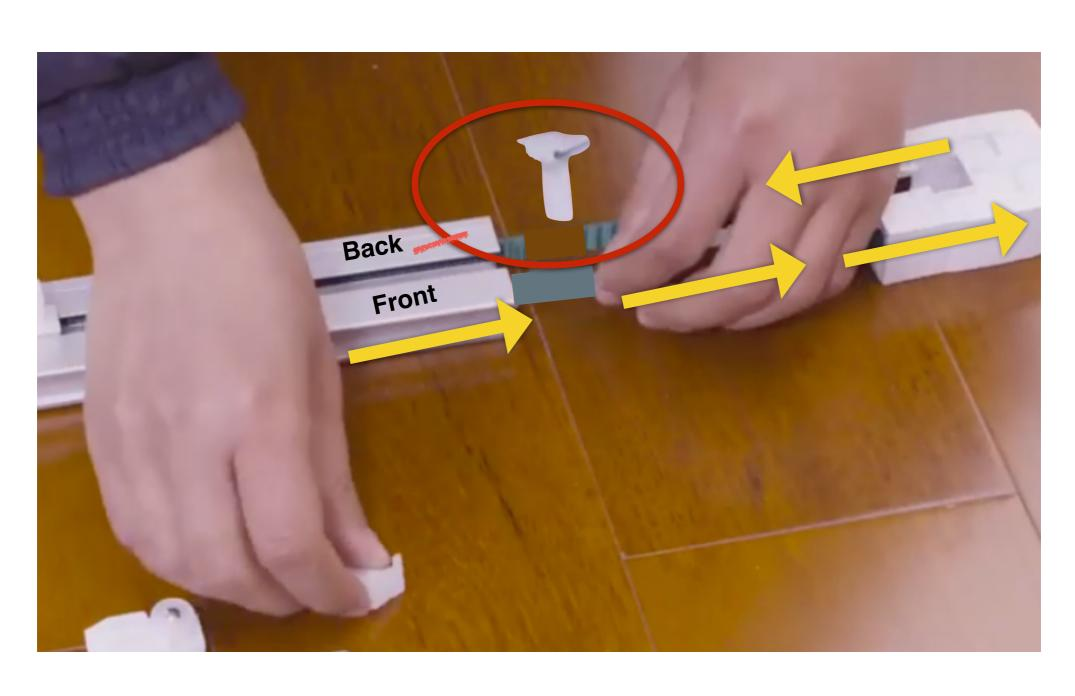
4. In this picture the buckle was inserted in the front of the rail, to reverse the open/close position the buckle must be inserted in the rear section of the rail
