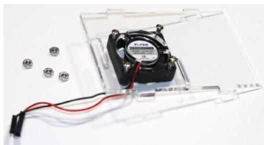
Drop in the 4 screws from the top so they pass through the acrylic and through the fan. Gently pick up the assembly while supporting the fan and not letting the screw come out, and put it at a slight angle so you can install the nuts on the back side of the assembly.
