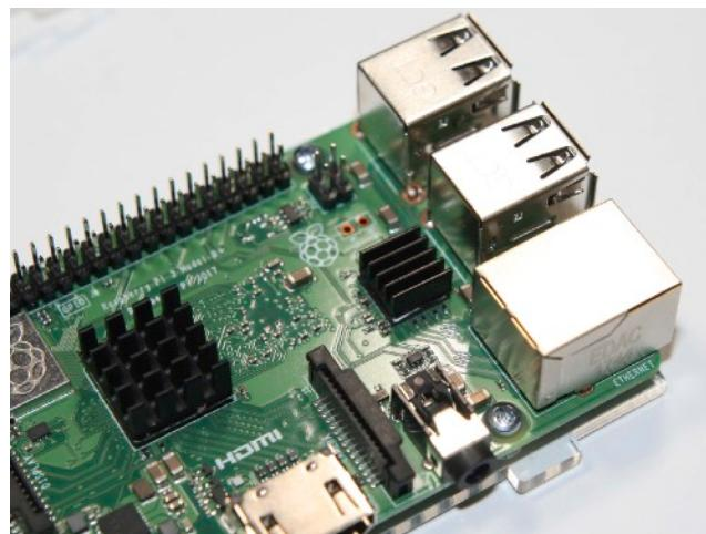
The smaller heat sink is for the USB controller (the next largest black chip on the top of the Pi). Remove the paper and stick it to the chip the same way you did the processor. Apply firm pressure to seat it. Your Pi should now look just like the picture. If it doesn't you messed up and should reread the instructions
