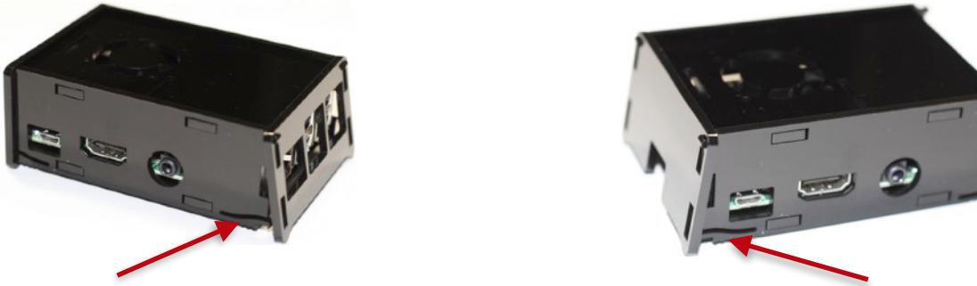
This is best done by holding the enclosure in both hands and pushing gently on the knurled areas on one side of the case. This will release the bottom "claws" and allow the cover to swing up enough that it can be gently removed from the top "claws." Do this for each side. Do not force anything. The "claws" can break if you put too much pressure on them.
