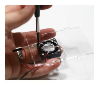
Use a Philips screwdriver to tighten the 4 screws. It helps to put a little pressure on each corresponding nut so that it doesn't turn while you tighten the screw. I'm not doing it in this picture because I'm holding the screwdriver and everything else with one hand while taking the picture with the other. I'm talented like that.
