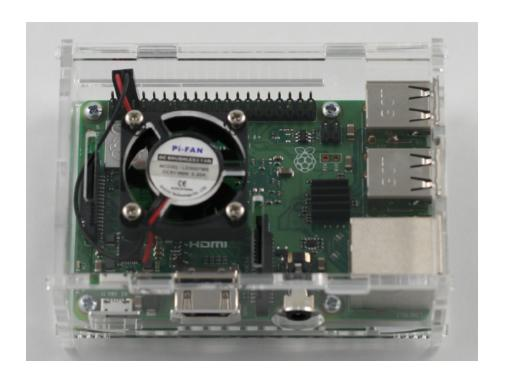
Finally, it's time to put the enclosure back together again. Do this the same way you took it apart but backwards. Make sure the wires do not get pinched in the case and are not touching the fan blade. Be sure you don't put too much pressure on the plastic "claws" when closing up the case.
