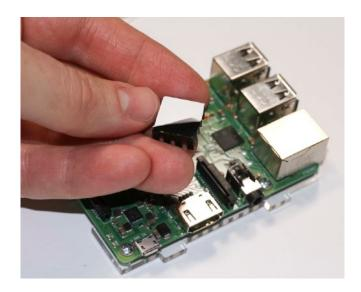
Put the top / fan assembly down for a few minutes while you install the heat sinks. The larger of the two heat sinks if for the processor. Grab it. Remove the paper backing from the adhesive and stick it to the center of the processor (the large, black or silver chip on the top of the Pi. Use firm pressure to seat it to the processor.
