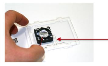
Place the fan onto a flat surface and orient it so you can read the wording on the front. Take the top piece of the enclosure and place it over top of the fan, paying attention to the orientation of the top piece. The camera connector slot should face you and be oriented exactly as it is in the photo.
