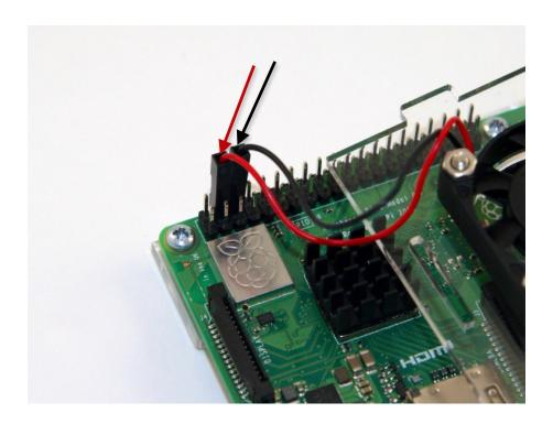
It's time to plug the fan into the Pi's GPIO for power. Pick up the fan / top assembly and connect the fan wires to the pins shown in the picture. Pay attention to the black and red wires. The red wire plugs into the 2nd pin on the top row from the left. The black wire plugs into the 3rd pin on the top row from the left. Pay close attention to the wires; if they are plugged in reverse the fan will not work. If they are plugged into the wrong pins the fan won't work.
