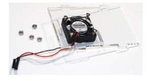
Drop in the 4 screws from the top so they pass through the acrylic and through the fan. Gently pick up the assembly while supporting the fan and not letting the screw some out, and put it at a slight angle so you can install the nuts on the back side of the assembly.
