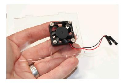
Thread the nuts onto the screws from the back of the assembly. Tighten finger tight.
