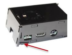
This is best done by holding the enclosure in both hands and pushing gently on the knurled areas on one side of the case. This will release the bottom "claws" and allow the cover to swing up enough that it can be gently removed from the top "claws." Do this for each side. Do not force anything. The "claws" can break if you put too much pressure on them.
