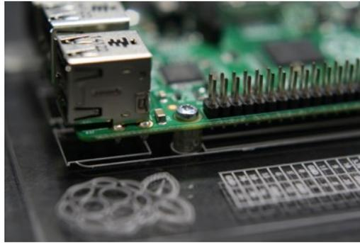
Using your small Philips screwdriver, screw the 4 screws until they are screwed snugly against the Pi. Make sure you don't over-screw the screws, just screw until the screws make contact with the circuit board.
