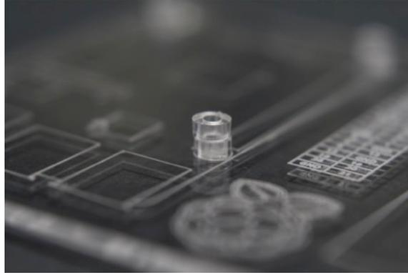
Flipping the plate back to the front and placing it on a level surface, stack 2 spacers on top each other on the appropriate holes for your Raspberry Pi (use the outer holes for a regular 40 pin Pi or the holes closest to the GPIO map for a Pi Zero.) Make sure you have all 8 spacers stacked over the holes. (2 spacers per hole, not one stack of 8 spacers, though I'm sure that would be impressive.)
