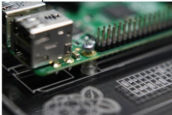
Line the Pi up with the laser cut outline and carefully lower it down on top of the plate, allowing the screws to go into the spacers. You might need to wiggle the screws slightly to make sure they drop all the way in.
