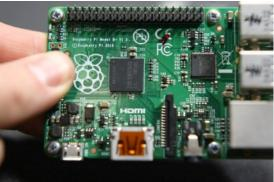
Hold the Pi with one hand and put the screws in each hole with the other.
