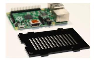
Center and place the four small spacers over the holes in the bottom plate. The Pi will sit on top.
