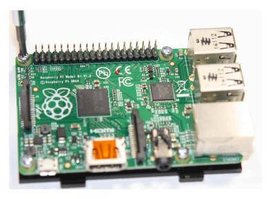
Put the screws in place and using your small Philips screwdriver, screw the 4 screws until they are screwed snugly against the Pi. Make sure you don't over-screw the screws, just screw until the screws make contact with the circuit board.
