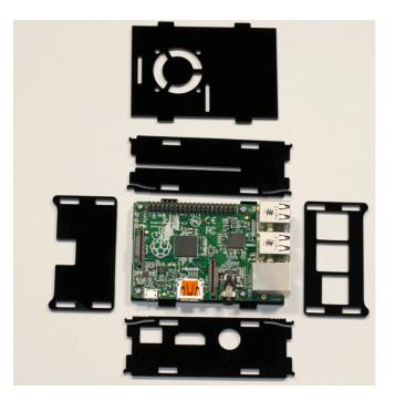
Align the rest of the parts as shown in the picture. Make sure the holes in the acrylic correspond to the ports on the Pi.
