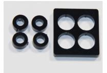
Next, pop out the four small spacers out of the acrylic square. If you have trouble, pushing the center of the hole with a screwdriver and poking them out works well.
