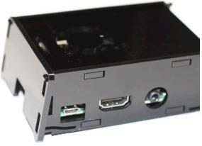
Now it's time to put on the left side. Make sure the cutout for the microSD card is on the bottom and "hang" the side from the top "claws" first. Once in place, you can gently push the bottom over the lower claw, snapping it into place. If it doesn't go easily it helps to wiggle the part from side to side to help it to snap into place.
