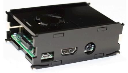
Being sure that the parts in the front line up with the ports on the Pi, put the front side into place. Remember to make sure the small slits that lead to the "claws" on the bottom.
