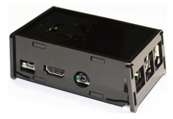
Do the same to the right side. The two taller holes line up with the two USB ports on the Pi. The smaller hole lines up with the Ethernet port. Once it's lined up snap the part into place just like the left side.
