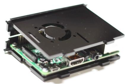
Put the top into place next. The vent holes go over top of the processor (near the Raspberry logo.) The slots correspond to the camera and CSI connectors. It might help to hold the top in place with your finger until the next part.
