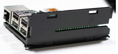
Put the back cover in place first. The slot should line up with the GPIO pins. The "ears" on the base will fit into the rectangular holes on the back cover. Be sure that the small slots that go to the little "claws" on the end are on the bottom.
