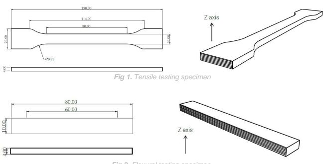
Fig 2. Flexural testing specimen
