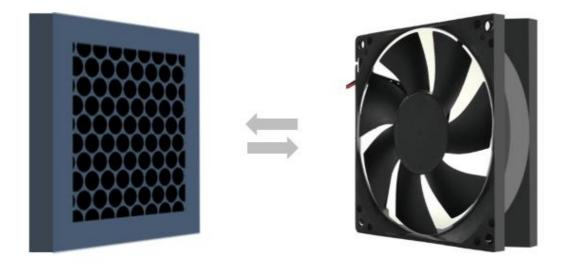
5. Hold the filter system with one hand and install the four Phillips head screws with the other hand. *Note:* Keep the tiny arrow on the label of the fan upwards. Be careful not to break the fan cable.
