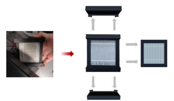
4. Take the original filter cartridge out and install a new filter cartridge.
