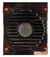
6. Install the Phillips head screws to the back cover.
