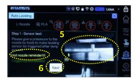
**STEP 4:** Clean the nozzle and the build plate, then adjust the Z axis with a leveling card with a thickness of 0.2mm according to the instruction on screen.
