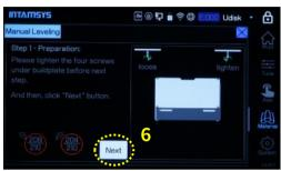
**STEP 4:** There are 4 screws which need to be adjusted one by one for at least twice, by using the leveling card with 0.2mm thickness.
