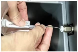
3. Insert the filament extension tube into the filament loading port. The filament preparation is finished and ready to print.
