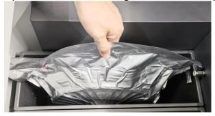
2. Gently pull out the filament from the filament extension tube, and insert it into the filament loading port.
