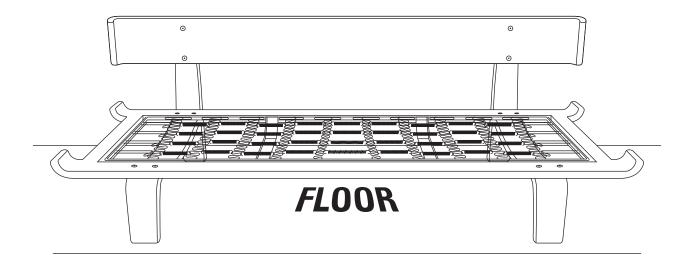
7 To attach the canvas spring cover, slide the elastic over the corners of the metal frame containing the springs. Done!
