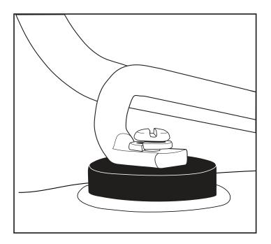
Thread all 4 screws lightly by hand to allow movement of base before tightening all 4 screws evenly with screw driver.
