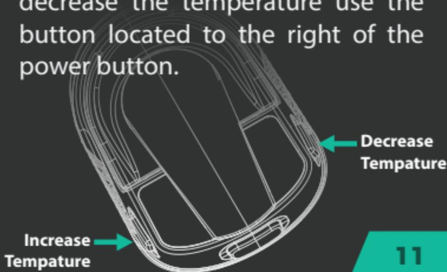
As before each single click will change the temperature, it will decrease the temperature by one degree. Temperature ranges from 104°F-428°F and 40°C-220°C. To switch between Fahrenheit and Celsius click the two side buttons at the same time once.
