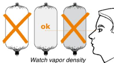
It is not necessary to fill the Valve Balloon completely. It is often sufficient to fill only half or even less than half of the Valve Balloon in order to achieve the desired results.
