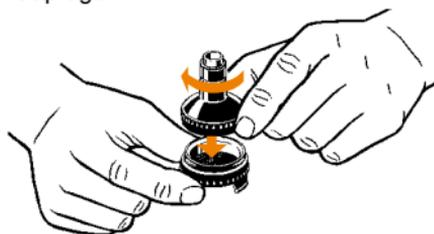
*Screw on Filling Chamber Cap*
