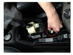
**04.** Disconnect shifter cables from the shifter base assembly, towards the front of the car.
