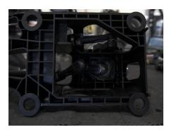
24. Re-Insert the shifter base bushings, and maneuver your shifter assembly back into its place in the car.
