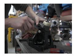
12. Lift out the metal shifter with attachments.
