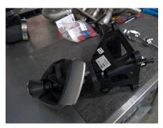
**07.** Punch out roll pin on front side of the shifter.
