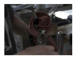
**15.** Next up you'll want to remove the stock shift knob. This can be a bit of a battle, but, it's a press fit knob so you'll need to use some force to pry it off. Your shift knob will most likely be completely destroyed in the process. Use whatever force necessary to remove, while keeping all other components intact.
