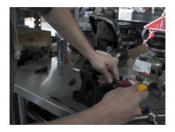
**09.** Pop off the 2 cable ends from underneath the shifter assembly.
