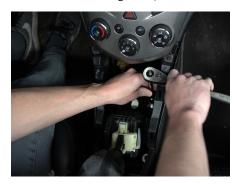
**06.** Pull the entire shifter assembly out of the car and to a clean, solid working area where you can begin swapping the shifter outside of your car.
