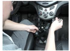
25. Slide the shifter linkages on to their mounts on the shifter base.
