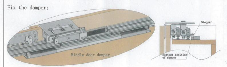
3. Install the stopper to the contact position of damper, adjust the middle door to the middle position, then fixing the damper by screw.
