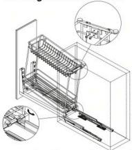
4.Fix the slice as shown and be sure slide moving smoothly.
