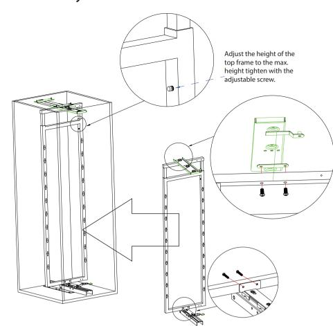
2. Fix frame onto the connector bracket on the top and bottom runner cover tighten with screw. Put the frame into the carcase rest on the top and bottom runner base.
