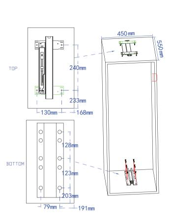
Fix top and bottom runner base according to the measurement stated above.
