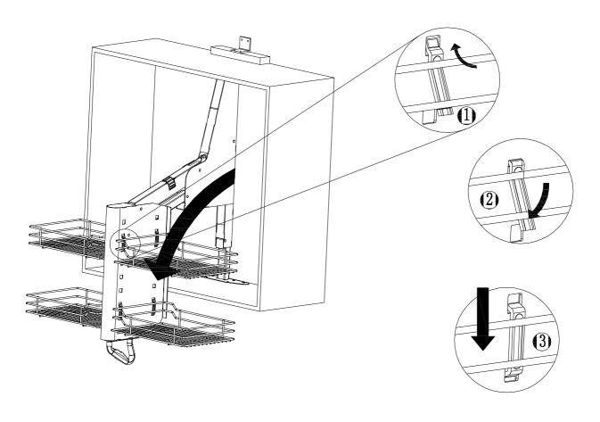
step 5: Adjust the product according to the heavyweight. The power buttom , you can adjust it when you screw out right or left. Attn: The best way you can adjust the power is when you push down the product to 90 degree.
