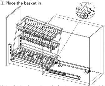
4. Fix the bracke as shown in the diagram. Be sure slide move smoothly
