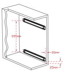
2) Lock the inner slide to the basket, then attach the outer slide to the slide as shown in the arrow diagram
