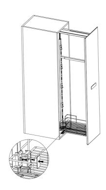
The graph shows the finished condition, and to ensure that the baskets are well installed, please press the edge of baskets to make sure that the edges are attached to the plastics fixed point (H).
