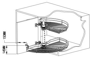
5. Connect the bottom basket with the the door bracket together as shown in the diagram.
