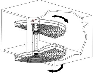
3. Fix the basket framework on the tube using the fixed base, and revovle freely as shown.
