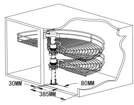
2. Fix the tube base into the inner cabinet with screws according to the diagram shown.
