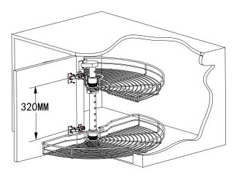
4. Fix the cabinet hinge and panel on the tube with screw according to the measurement shown.
