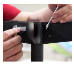
4. Using a 7/16" ratchet and 7/16" wrench tighten every bolt and nut.
