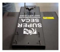
3. With a Philips screwdriver tighten the screws slowly. DO NOT over tighten them.
