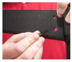
1. Line up the holes of the leg with the holes on the bottom of the lower tube and insert two hex bolts.
