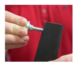
5. Install each leveler an equal distance from the bottom of the leg to ensure base stability.
