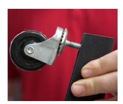
6. To install the optional caster system, thread the caster completely into the bottom of the leg.
