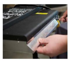
3. Place the second skirt on either side of the element. First, thread the screw at the end in order to leave room for adjustments. Thread the other two screws into the top of the skirt.
