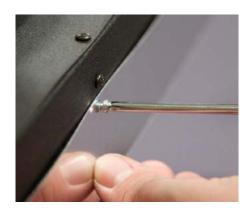
2. For the middle skirt, thread the middle screw first. This allows for room to adjust if needed. Thread the other two screws into the top of the skirt.
