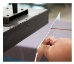
1. Start with the middle reflective skirt, place it against the heating element and align the holes of the skirt with the holes of the element.
