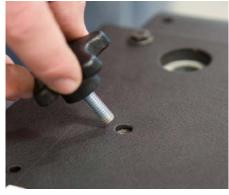
5. Install the angle adjustment knob into the threaded hole on top of the plate.
