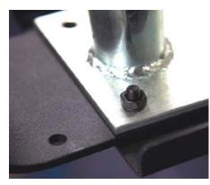
4. Screw on a lock washer and a nut to the other end of the bolt. Repeat to the other side. At this point, both of the bolts should only be tightened by hand.
