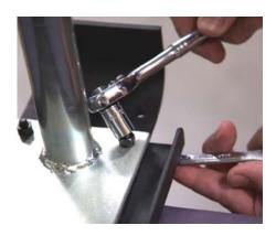
6. With a 7/16" ratchet and 7/16" wrench tighten the two bolts. The inner tube and top plate are now assembled.
