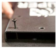
2. Place eight mounting screws into every hole except for the very top middle hole.
