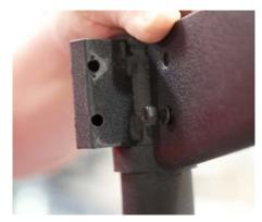
2. On the other side of the leg thread a lock washer and a nut onto the opposite end of each bolt.
