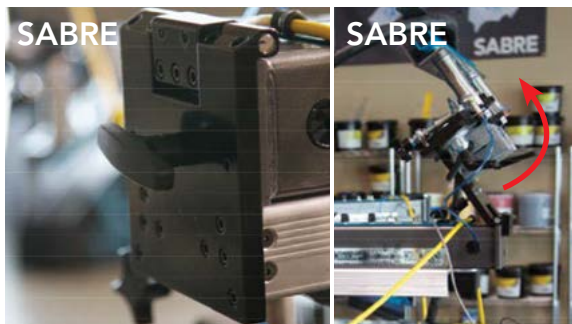
SABRE - Loosen the T-knob and pull the hinged front screen clamp up and over the top of the print head.
