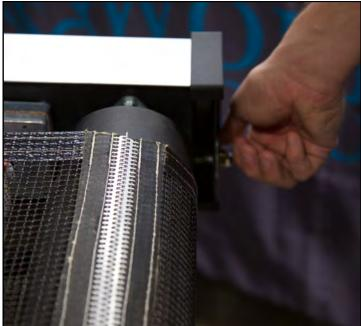
After the belt is centered on the rubber portion of the rollers, evenly adjust the tension bolts on every corner of the dryer to tighten the belt until it can be deflected by about 2 inches. Turn the dryer on and set the belt speed to 35%, as the belt moves make small adjustments to maintain the belt to be in the center of the rollers. Turn the tension bolts clockwise to tighten the belt in that corner, or turn the bolt counter-clockwise to loosen the belt in that corner.
