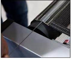
5. Align the belt closure until the teeth mesh connect, and install the fasting pin into the teeth. Hold together the teeth while installing the pin. When it's inserted and the belt is fully installed, trim any extra pin that may be jutting from the sides.
