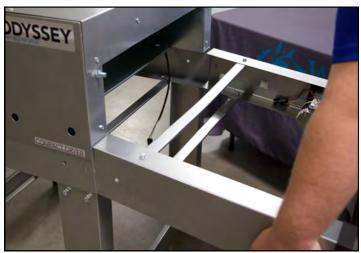
1. The side with the wire is the side that the outfeed is installed into. Slide the arms (with the motor) into the base, while aligning the holes of the arm and the base.
