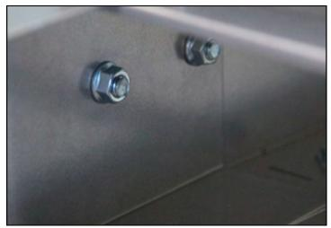
3. Thread a lock nut onto the other side of the bolt, which is located inside of the dryer. Repeat steps 2-3 to install the other three holes. Do not tighten the nuts and bolts with wrenches until the belt is installed.
