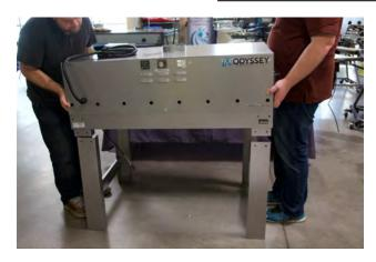
6. Set the legs up so the outsides of the cross braces are facing out. Using two people, lift the dryer body and insert the bottom corner slots into the legs.
