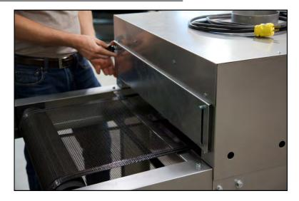
Test the first dried garment with a non-contact infrared digital thermometer. Adjust the belt speed to achieve the desired ink curing temperature.
