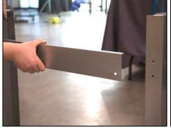
1. Align the holes of the cross base with the holes on the bottom of two legs. The backside of the cross brace should face out, and the inside of the brace should face in.
