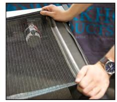
3. Thread the belt until both ends meet on the outfeed roller.
