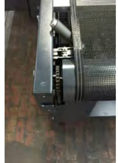
Belt motor chain to see if broken (take guard off to access). Replace if necessary.
