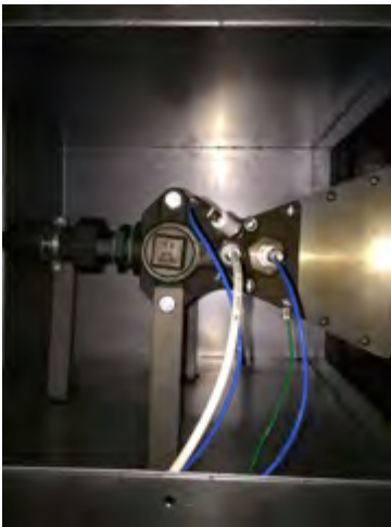
Igniter (white wire), check wire condition and fitting connection. If it is brittle and cracked, replace it. Remove spark plug and clean gap at the tip of the spark plug using fine sand paper.
