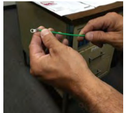
5. Inspect ground wire (green wire). If it is brittle and chipped, replace it and be sure it grounded to the basket.
