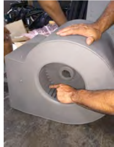
2a. Thoroughly clean recirculation blower
