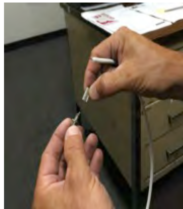
Fitting connection instruction: -Unthread connector into two pieces -Strip end of igniter wire back 3/16" -Insert stripped wire into top portion of fitting and thread two pieces back together
