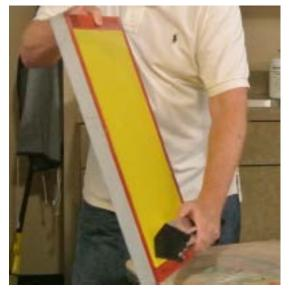
It's important to coat the outside (print side) first because it will leave a heavier deposit on the screen.
