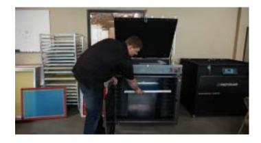
A Workhorse SD-10 drying cabinet will speed up the drying process and eliminate the danger of dust, which will guarantee high quality screens and increase production speed.
