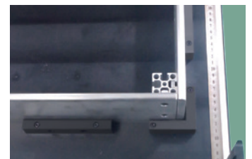
Locating Blocks and Pusher Frames
