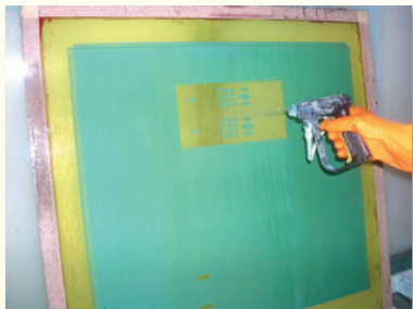
Step 1. After removal of ink, block-out, and tape, apply Gem-Zyme to a wet screen(both sides).
