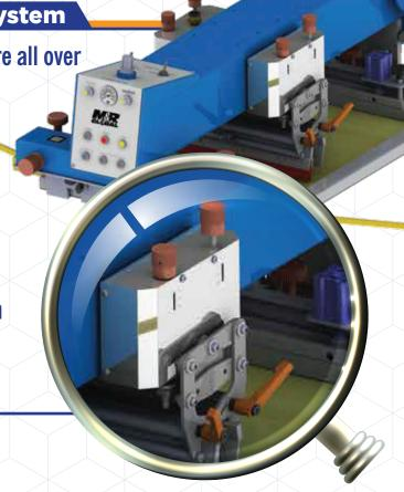
Individual mechanical head lifts assist operators for quick and easy screen cleaning
