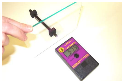
STEP 3: → UV Transmission Measurement shown with coated glass sample
