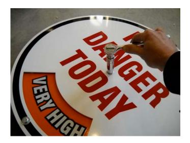
Be sure to not over tighten center mounting lag screw. Color wheel should turn without resistance.
