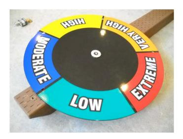
Place the color wheel on the post aligning the center hole. (Do not attach.)
