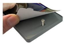
The front panel membrane has two tabs that can be flexed outward to allow access to the panel fixing screws. Once fastened in position and tested the backing paper can be peeled off and the tabs fixed down flush to conceal the screws. ONLY perform this operation once the installation has been tested and found to be satisfactory.
