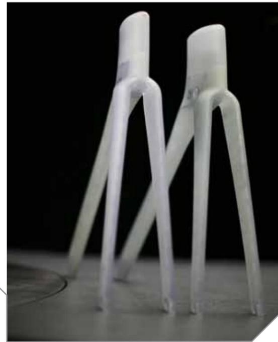
3D printed SLA prototypes
