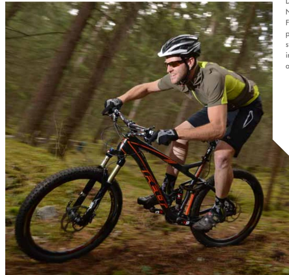
Felt engineers understood that there are typically two methods for increasing stiffness of a carbon frame. Add more material or add higher modulus material. But both strategies have downsides. Higher modulus material is more expensive and more brittle. Extra material means a heavier bike.
