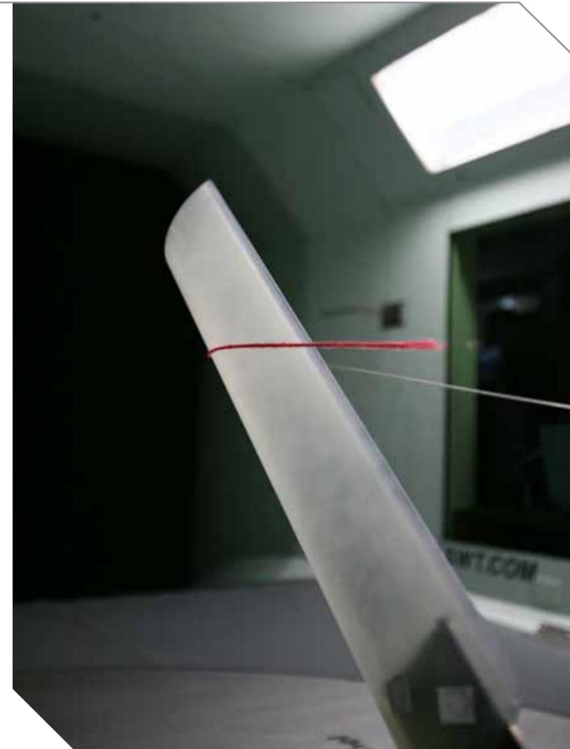
Testing a section for a downtube for aerodynamic efficiency
