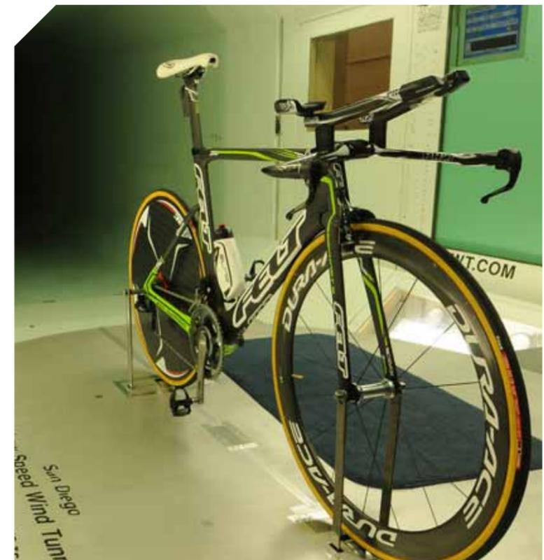
This is key. Instead of wind tunnel tested, Felt aero bikes are wind tunnel developed. We are bringing prototypes to the wind tunnel, making changes, and then going back and refining the design before the carbon fiber molds are ever cut. There is a big difference between sticking a finished bike in the wind tunnel and blowing air at so you can say you were there, versus multiple trips making changes, before you finalize the design.
