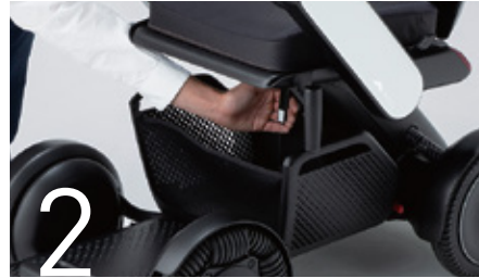
2 Raise the lever under the seat.
