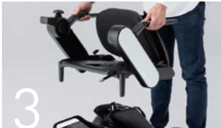
3 Pull the seat upwards.
