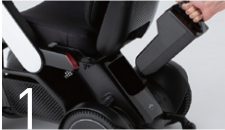
1 Remove the battery.
