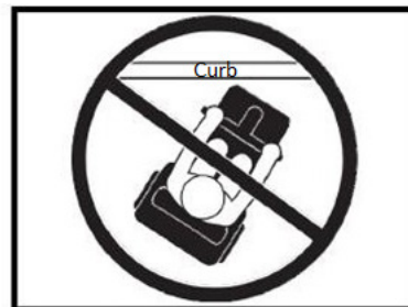
incorrect curb approach
