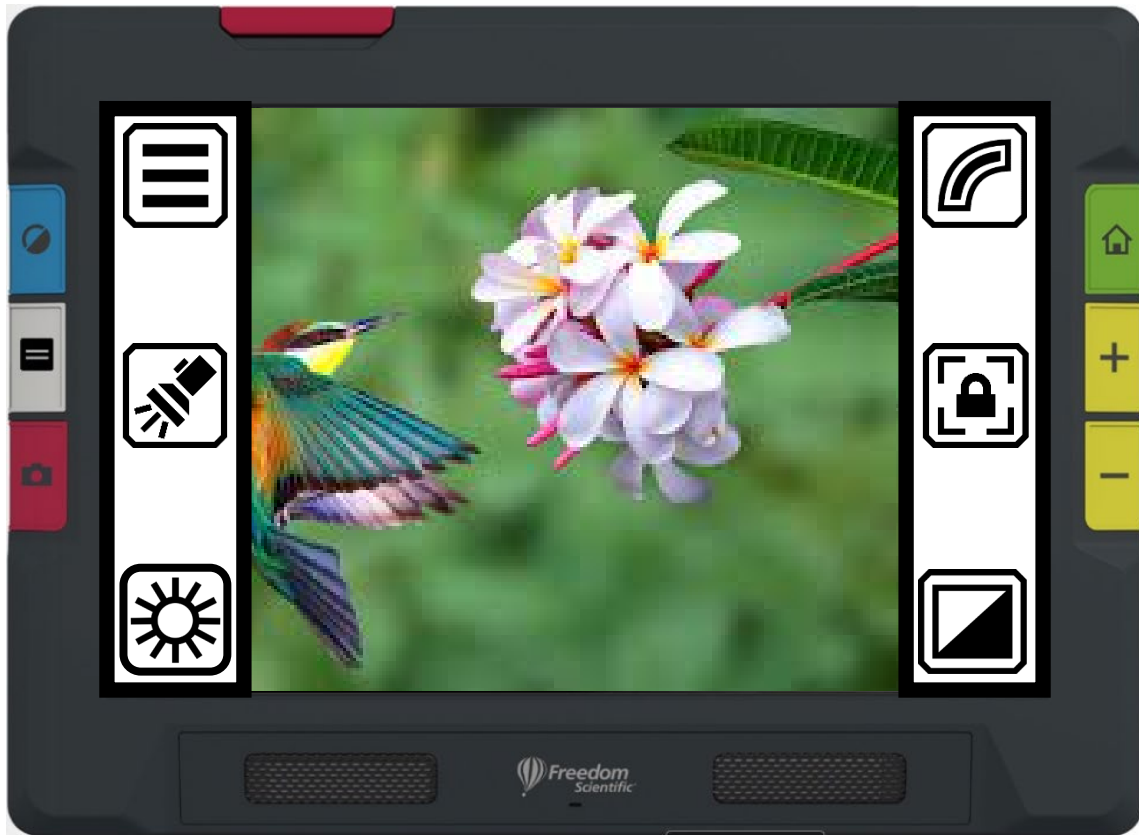
Sample showing the buttons that display while using the Overview camera in Advanced mode
