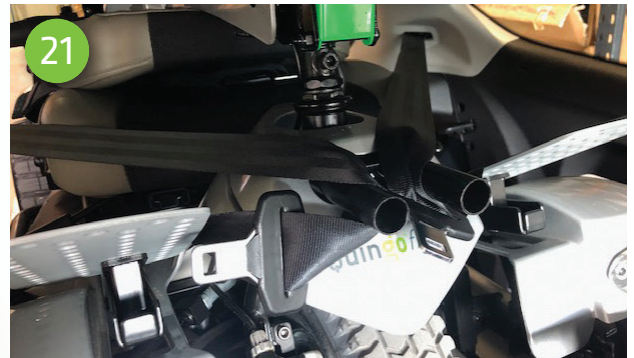
21 Go to the side doors and pull from each side the seat belt and locate the seat belt around the front basket bracket. Repeat this each side.
