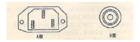
For charging, just insert the charger plug into the charging socket of the battery as shown in Fig. A and Fig. B.
